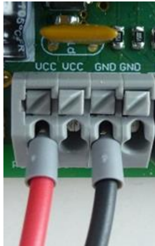
Figure 39: Terminal block for the power supply
