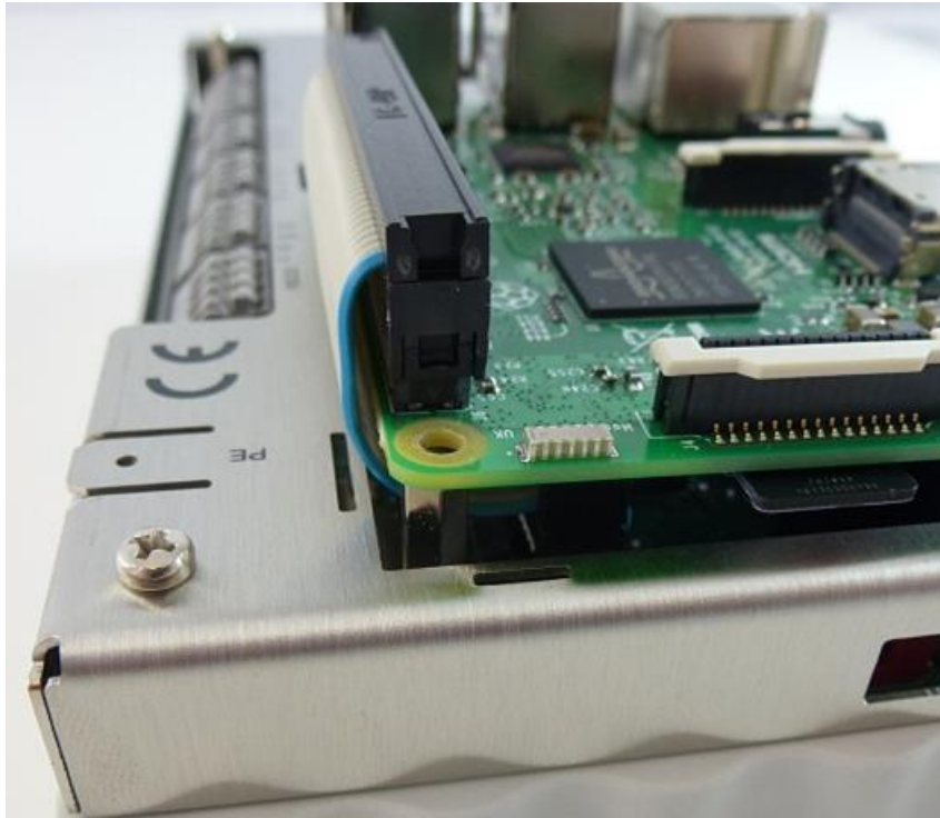
Figure 23: Optimal routing of the ribbon cable
