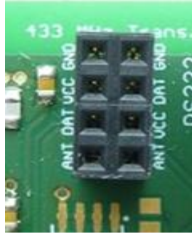
Figure 73: Two-row socket connector for 433 MHz transmitters
