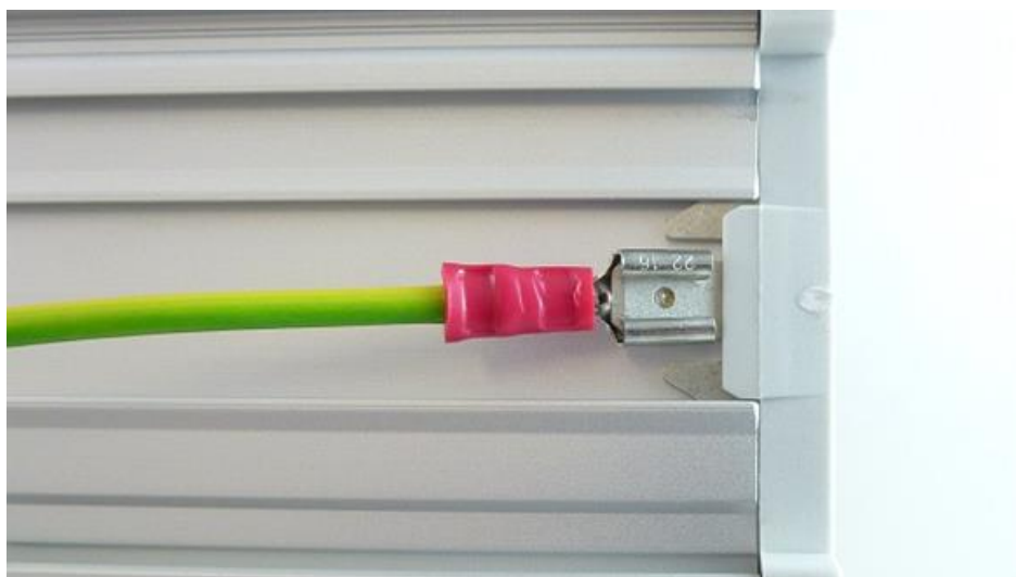
Figure 16: DIN rail housing with grounding connection (PE)
