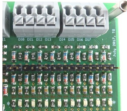
Figure 52: Terminal block - digital inputs
