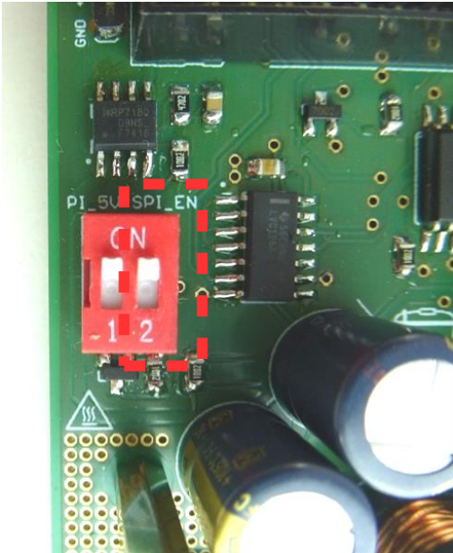
Figure 47: DIP switch: SPI_EN
