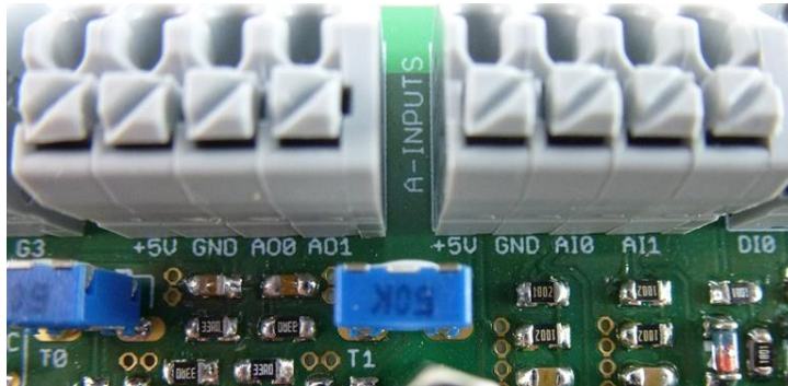
Figure 63: Terminal blocks - analog inputs and outputs
