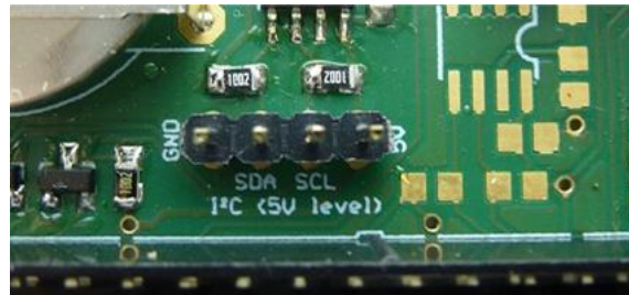
Figure 43: Pin header - I 2 C on 5V level
