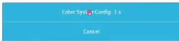
Through this, the most important parameters (URL address of the web server, IP address, browser display mode etc.) can be configured. This web configurator can also be accessed via a web browser on another device connected to the Web Panel via a network cable.
